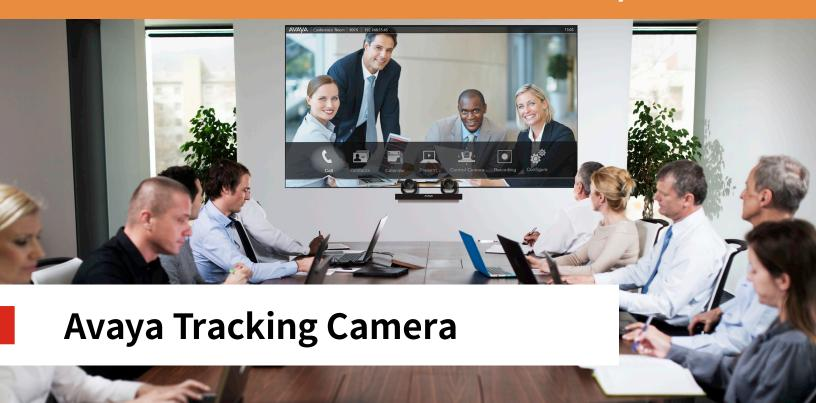
Avaya Tracking Camera is a smart solution for large meeting rooms, directing the meeting in an intelligent way, by focusing on an active speaker. With the combination of audio tracking and face recognition, it properly identifies the active speaker (or speakers) position, and the dual cameras handle the transition from one view to the other fluidly.
